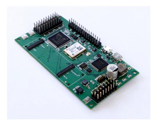
The AeroCore runs the NuttX real-time OS on a ARM Cortex-M4 microcontroller, with space on board for
