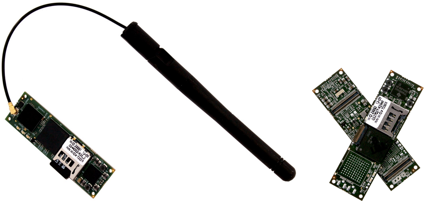
The Gumstix DuoVero Zephyr COM with WiFi antenna (left) and Overo TidalSTORM COM (right)
