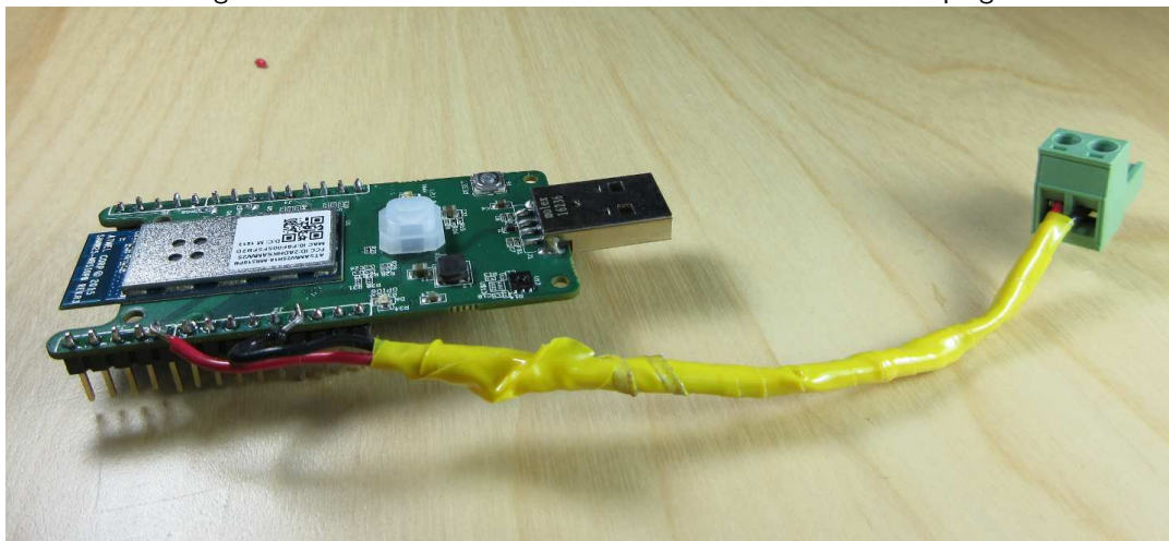
Figure 3: RoomSense with wires connected to screw-terminal plug
