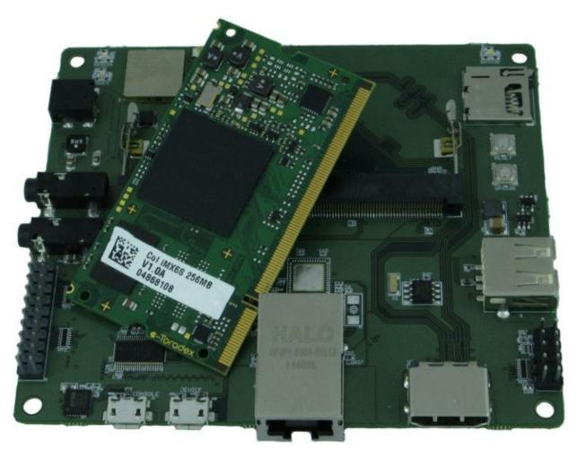
The Gumstix Colibri i.MX6 Dev Board is a multifunctional testing platform for the Toradex Colibri i.MX6 SOM with a wide array of multimedia I/O as well as GPIO, SPI and I2C headers.
