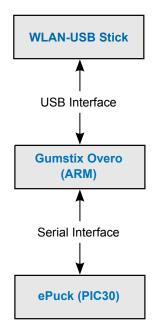
Fig. 2. System structure of the ePuck robot
