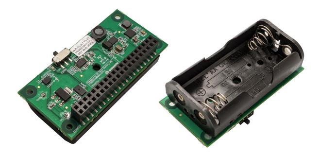
The <u>Gumstix Raspberry Pi Zero Battery</u> IMU board allows you to take your Raspberry Pi Zero anywhere. Simply pop in two rechargeable NiMH or NiCd batteries into the holder and you're ready to go with your Raspberry Pi Zero. Charging the batteries is as easy as plugging in your Raspberry Pi Zero using a USB cable, as per usual. With the onboard Bosch BMI160 3-axis accelerometer and 3-axis gyroscope you can easily track motion. Add a camera to enable totally wireless video streaming.
